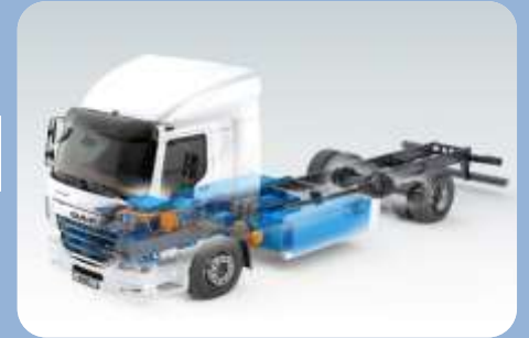
Battery Thermal Management System
